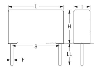
StyleRadialFeaturesAutomotive Grade, PulseRoHSYesTerminationTinned WireLeadWire LeadsQualificationsAEC-Q200AEC-Q200Yes
