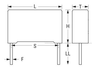
R76 Series Dielectric **Double Metallized** Polypropylene Style Radial Features Pulse RoHS Yes Cut (Tinned Wire) Termination Lead Cut AEC-Q200 No 5.88 g **Typical Component Weight**
