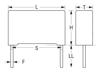
Dielectric **Double Metallized** Polypropylene Style Radial Pulse Features RoHS Yes Tinned Wire Termination Lead Wire Leads AEC-Q200 No **Typical Component Weight** 8.45 g
