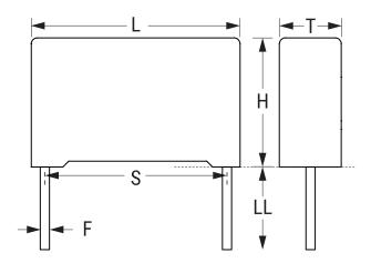
StyleRadialFeaturesPulseRoHSYesTerminationTinned WireLeadWire LeadsAEC-Q200NoTypical Component Weight7.9 g
