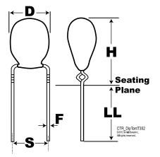
**General Information** T352 Series Dielectric MnO2 Tantalum Style Radial Description Radial, Solid Tantalum, Conformal, Dipped Low Leakage Features RoHS Yes Termination Tin AEC-Q200 No Construction Conformal Notes Longest Lead Is Positive.
