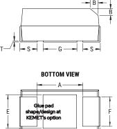
Description SMD, MnO2, Molded, Low ESR Features Low ESR RoHS No Prop 65 WARNING: Cancer and reproductive harm https://www.p65warnings.ca.gov SCIP Number 1dd2e1b8-26dd-4d52-927c-6f9 d519011aa Termination Tin Lead (SnPb) AEC-Q200 No **Typical Component Weight** 107.45 mg Shelf Life 156 Weeks MSL 1
