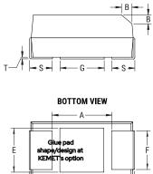
Style SMD Chip Description SMD, MnO2, Molded, Fused Features Integral Fuse RoHS No Prop 65 WARNING: Cancer and reproductive harm https://www.p65warnings.ca.gov SCIP Number 1dd2e1b8-26dd-4d52-927c-6f9 d519011aa Termination Tin Lead (SnPb) AEC-Q200 No **Typical Component Weight** 446.84 mg Shelf Life 156 Weeks MSL 1
