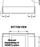
For T520 Series, bevel is at KEMET's option В
