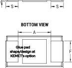
For T520 Series, bevel is at KEMET's option В
