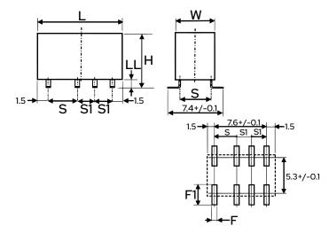
General InformationSeriesUB2StyleSMDDescriptionMiniature Signal Relay, Single<br/>Coil LatchFeaturesSuper-Compact Size, Flat-<br/>PackageRoHSYesCoil TypeSingle Coil (Latching)
